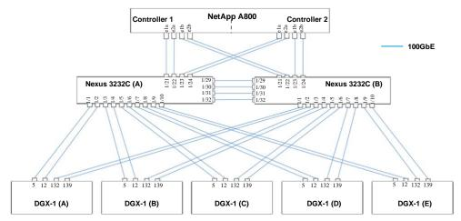
With A700s, the architecture shown in Figure 1 changes to a 1:4 configuration (1 A700s : 4 DGX-1), with four 40GbE links from the A700s to each switch on the storage side and two 100GbE links from each DGX-1 to each of two switches. In addition to 100GbE, the A800 system also supports 40GbE. Both architectures can scale up and out with zero down time as the datasets grow in size.
