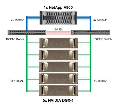
Figure 2 shows the port level connectivity of the architecture. This architecture consists of two Cisco Nexus 3232C 100GbE switches as well as a 1GbE management switch (not shown). There are five DGX-1 servers connected to the network with four 100GbE links each, with two links from each DGX-1 connected to each Nexus switch. Storage is provided by a NetApp A800 HA pair, with each of the two storage controllers connected to each Nexus switch with two 100GbE links.
