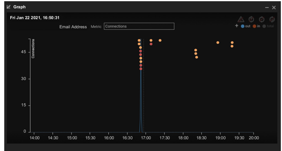
Figure 8: The connections associated with the compromise are a significant deviation from the device's normal 'pattern of life' and results in multiple unusual activity events and repeated model breaches (orange).
